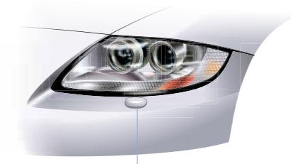
Complex optical system with automatic level control and power-wash system
